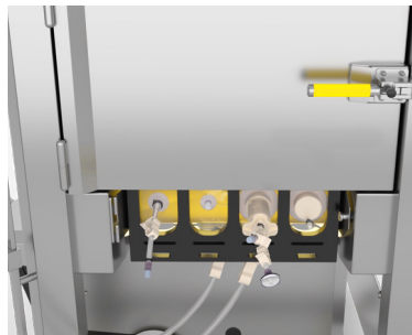
Front access to sensors and tubing for easy manipulation
