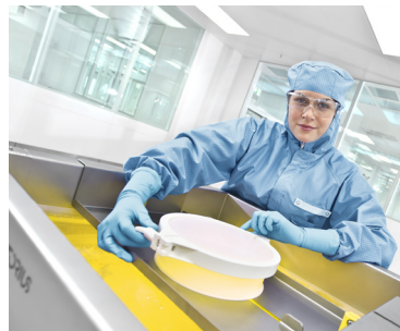
8 inches top opening for easy powder addition
